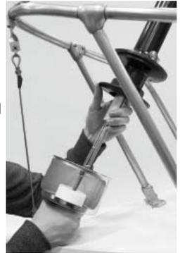
13. Pass the furling line through the hole in the side of the cup, then up through the hole in the top of the furling drum flange. Tie an overhand knot to prevent it from escaping.
