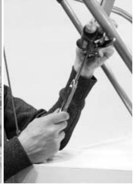
Screwing turnbuckle on stud.
