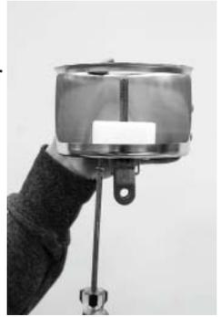
11. Slide the furling drum over the luff with the sail feed slot on the same side as the tack anchor shackle (see drawing above). You may knock the thrust washer (part “K” on page 2) out of place doing this. You can push the washer up into the cavity of the furling drum again. The washer is designed to ride between the furling drum and the bearing.
