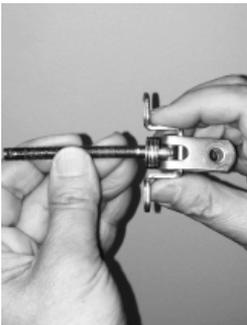
10. Select the appropriate pair of holes (on the bottom of the cup) based on the orientation of the chainplate and furling line. (See page 10 for more information.) Then screw the antirotation strap, bearing and cup together.
