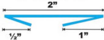
**Two layers of 2" facing makes a vertical or horizontal zipper cover**
