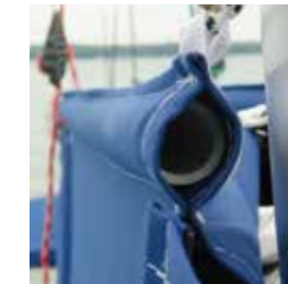
Sleeve opening for PVC pipe to keep cover open when lowering sail.
