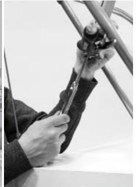
Screwing turnbuckle on stud.
