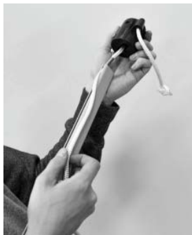
Pull halyard thru HTF. Ferrule gets inserted into the top of the luff extrusion.
