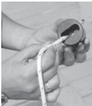
Feed halyard into bottom of HTF and out the side
