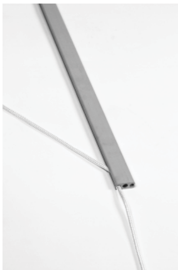
Pull halyard thru HTF. Ferrule gets inserted into the top of the luff extrusion.
