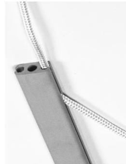
4. A) Using the de-cored (hollow) end of the halyard with the metal ferrule, pass the ferrule down through the slot at the top of the luff extrusion on the opposite end of the sail feed slot. Trimming the halyard to the correct length will happen once the entire furler is setup.
