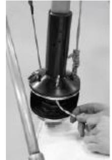
18. Use a furling line (not included) to go through the opening in the cup and up through the hole on the top flange of the spool, tie a knot to secure the line in place.
