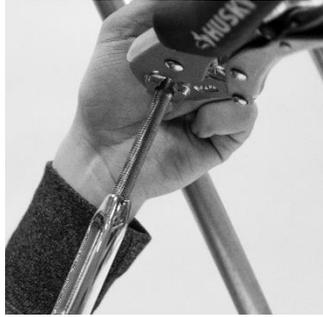
9. Using your T-bolt, add additional washers to reduce the clearance between the T-bolt and the bottom of the cup.
