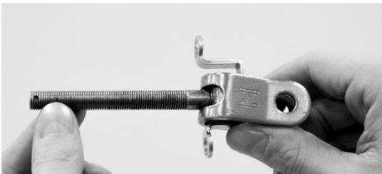
11. Place the T-bolt and the anti-rotation strap through the bottom of the cup, then add the bearing (plastic or ball-bearing) to the T-bolt on the inside of the cup.
