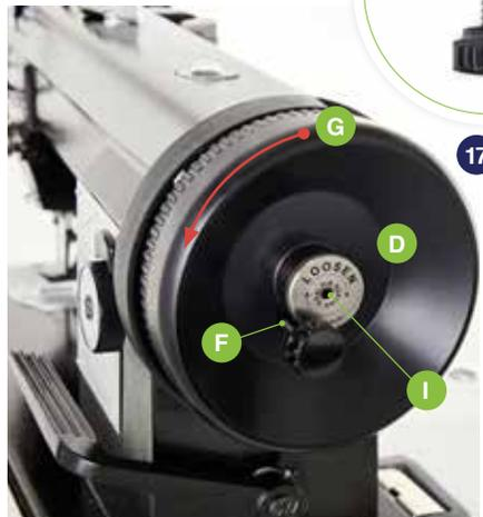
Push the Posi-Pin® (16) through the hole in the balance wheel (F). While maintaining pressure on the Posi-Pin, rotate the balance wheel (G) until the Posi-Pin locks into one of the balance wheel bushing holes (H). Rotation of the balance wheel will now cause the machine to function.
