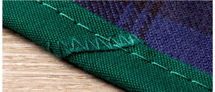
When you're sewing binding or welting with a splice onto a project, you don't need to do anything differently. The material will still fit through a binder attachment, such as the Sailrite® Swing-Away Binders. Just feed the material through the binder and sew it on as normal.
